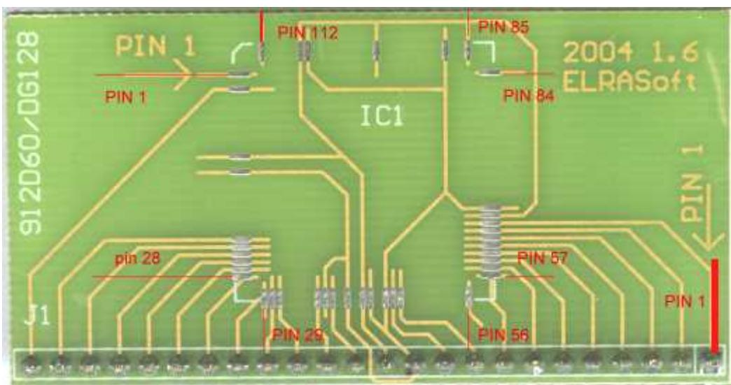
Check for shorted pins by an ohm meter
