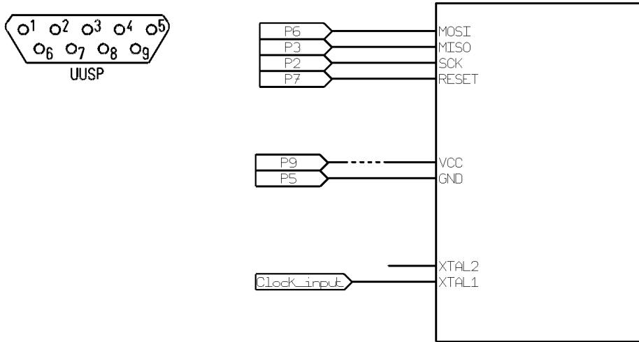
Either an external clock is supplied at pin XTAL1
